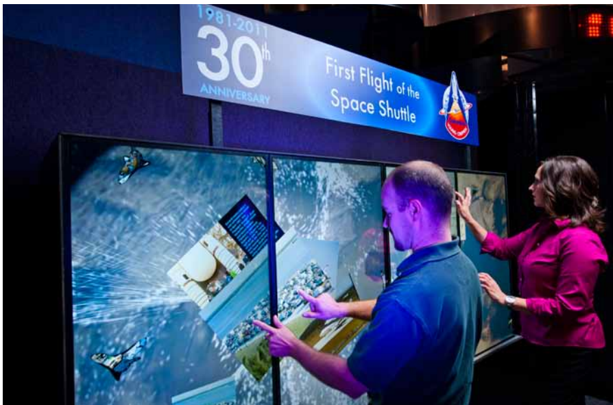
The interactive video wall at the Space Center Houston Visitor Center is made of four 46-inch MultiTouch Cell displays.
