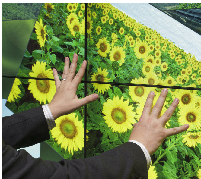
World's first ultra thin bezel LCD in an interactive display allows near seamless video walls of up to 24 units.
